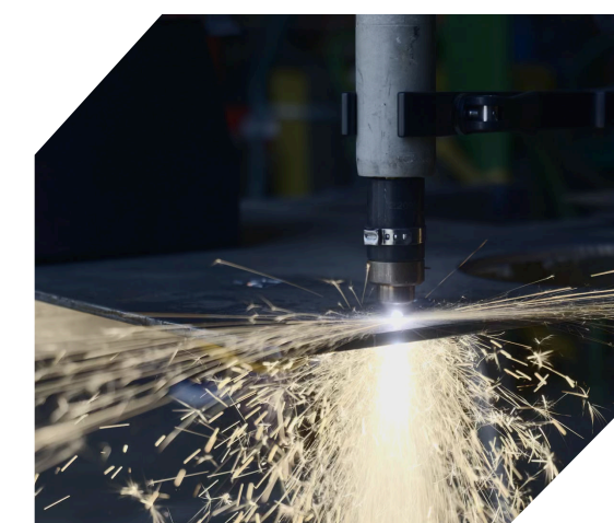
Mach 1 Plasma Cutting with Torch Height Control
